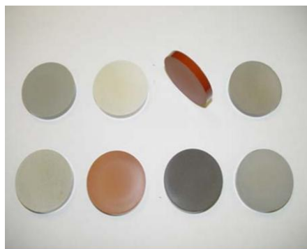
Figure 24: Example of pressed pellets prepared using 120 g of sample and 3 g of Pellet Blend Binder
