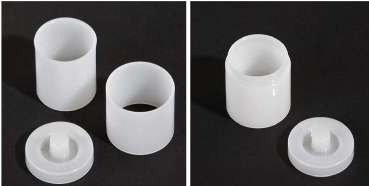
Figure 19: left: 35mm sample cup shown in the three individual pieces prior to assembly. right: 35mm cup assembled and ready for sample introduction
